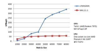
Figure 10: Performance of clMAGMA's Cholesky factorization in double precision vs. MKL 11.1
