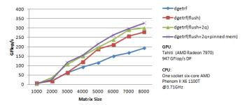
Figure 8: Advanced performance optimizations of dgetrf in clMAGMA.
