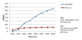
Figure 9: Performance of clMAGMA's LU factorization in double precision vs. MKL 11.1
